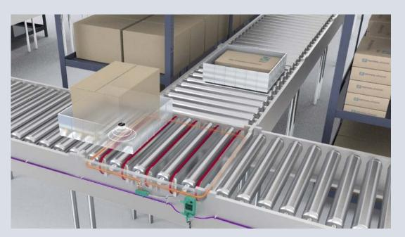
Conveyor systems based on ethernet solutions that support topology detection can make use of the switch build into the IDENT Control interface to automatically determine the conveyor layout.
