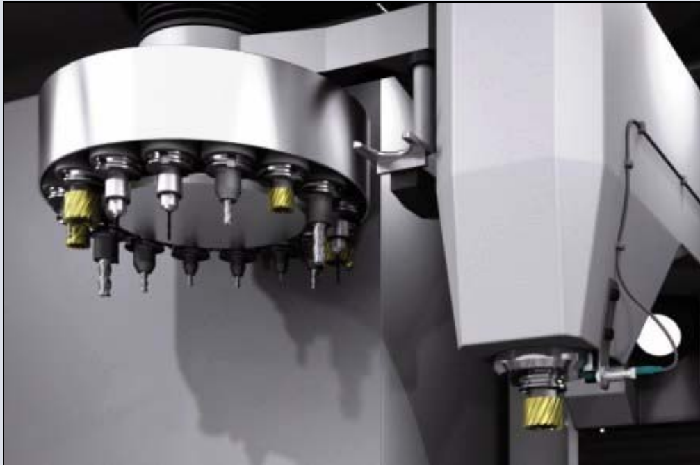
An RFID system enables this automatic tool changer setup to securely pick the right tool for the job.
