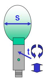
Regarding to the formular v = s/t the possible maximum velocity is calculated out of the size of the reading field and the execution times of the operation (see above figures).
